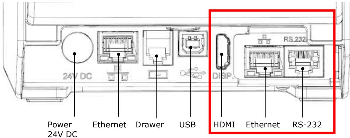
Connectors marked with a frame appear depending on the fiscal printer configuration. It is possible that the user will not have an additional Ethernet or HDMI connector.
