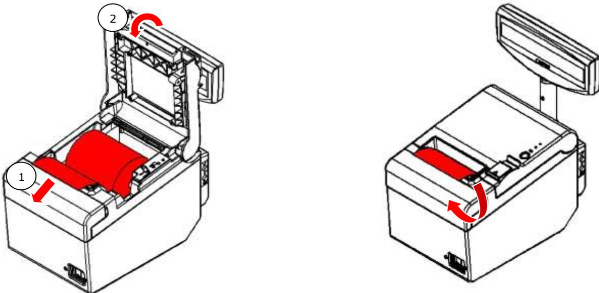
In the event of replacement of a roll into a new one, note that the remaining of the waste paper roll should be removed.
